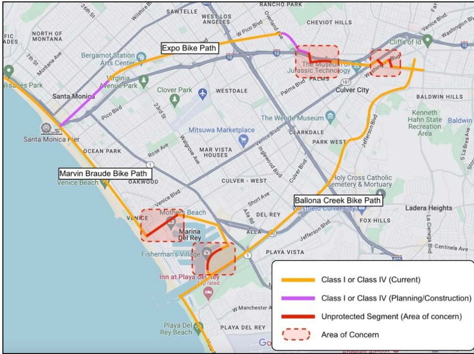
Figure 1. Fully separated or protected bike paths form a westside loop of connectivity, but areas of concern limit all-ages/all-abilities accessibility. The Marvin Braude Bike Path, Expo Bike Path, and Ballona Creek Bike Path contain short high-stress sections. Some are being addressed: Santa Monica’s Broadway and Colorado Ave protected bikeway projects will connect the Marvin Braude and Expo Bike Paths and will begin construction in 2024. LADOT’s Northvale Segment project will resolve a gap in the Expo Path between Overland Ave and Motor Ave and is beginning construction in 2024. Other gaps include on Washington Blvd and Fiji Way in Marina Del Rey, Downtown Culver City, and on Motor Ave and National Blvd in Palms. All areas of concern other than Fiji Way are included in the Los Angeles Mobility Plan as Class IV bike lanes.
