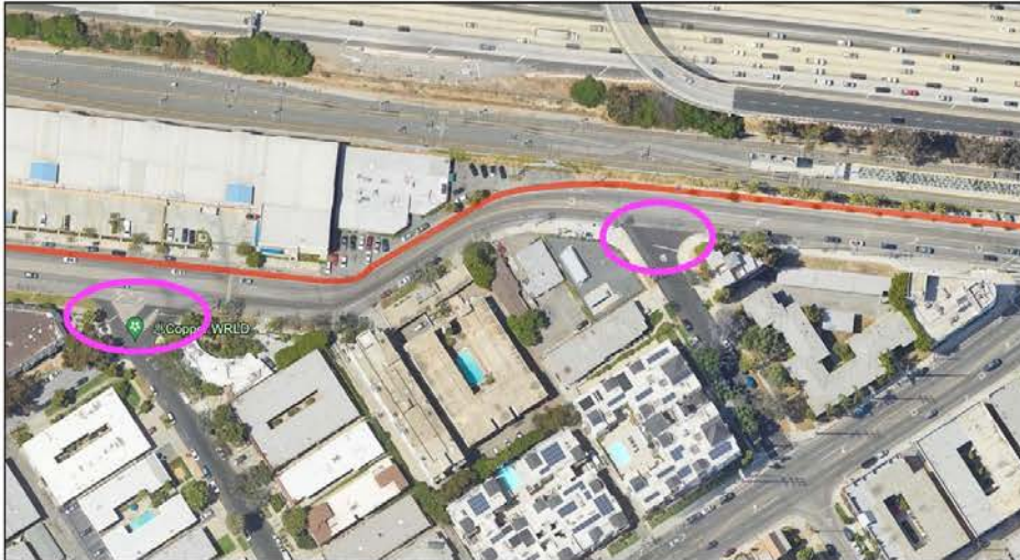
Figure 5. Alternative 1 increases safety by avoiding vehicle points of conflict. Alternative 1 would utilize a new signal and crossing, already included in the Northvale Gap Closure Project, to access a two-way cycle track on the East side of Motor Ave and continues on the North side of National Blvd. At Irene St, Vinton, Jasmine Ave, and Clarington Ave, dangerous geometry allows high-speed turns by vehicles, but all are avoided in Alternative 1. Additionally, a currently dangerous left turn by bicycle from Motor to National is avoided in Alternative 1. The result is an Expo Bike Path that is appropriate for all ages and abilities.
